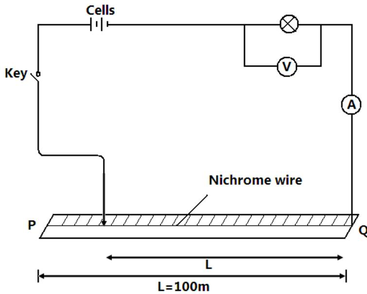
ii) With the crocodile clip at p, take the voltmeter reading and ammeter reading. Record v and I repeat the readings for L=80, 60, 40, 20 and 0cm respectively and complete the table below.
