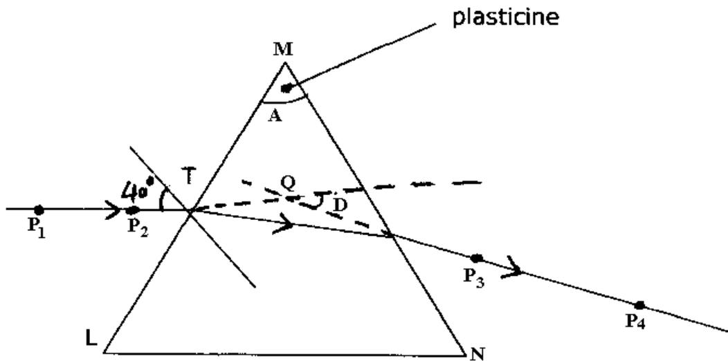
ii) Measure angle A of the prism using a protractor.
