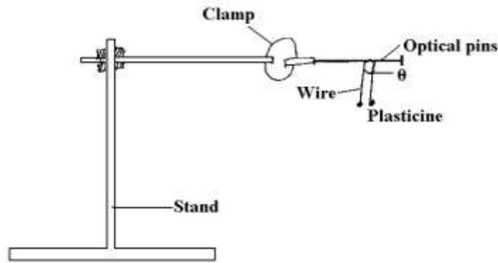
b) Bend the wire in the middle so as to make an angle of  $50^\circ$ . Attach the two small pieces of plasticine at both ends of the wire as shown in the diagram.
