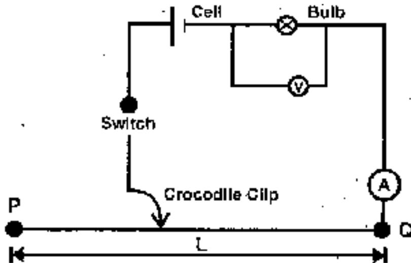
(ii) With the crocodile clips at P (ie  $L = 100\text{cm}$ ) take the voltmeter reading ( $V_0$ ) and the ammeter reading. Record  $V$  and  $I$ . repeat for  $L = 80, 60, 40, 20$  and  $0$  cm respectively.
