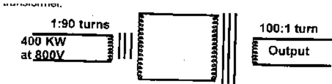
The generator produces 400kw at 500v which is fed into transformer T1 whose primary to secondary turns ratio is 1: 90
