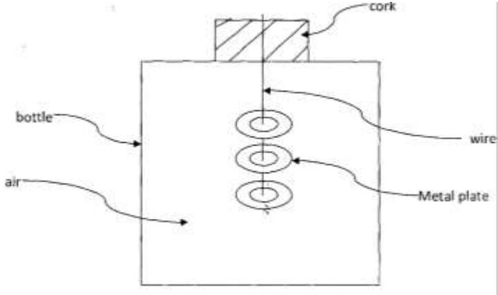
It is observed that when the bottle is shaken sound from the metal plates is heard. State and explain the observation that would be made if a little hot water is poured into the bottle then the cork is tightly replaced and the bottle shaken. (2 marks)
