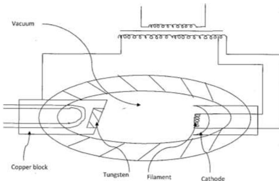
(i) Why is a thick copper block used at the anode? (1 mark)
