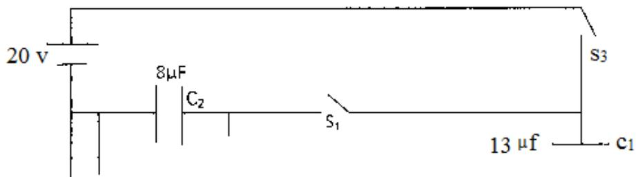
(i) Determine the charge on  $C_1$  when switches  $S_2$  and  $S_3$  are closed while  $S_1$  is open. (2 marks)
