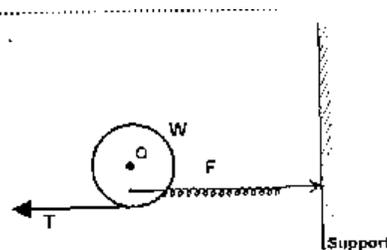
Figure 5 shows a wheel W pivoted at its centre O and held station by a string and a spring. The tension in the string is T and the force on the spring is F.
