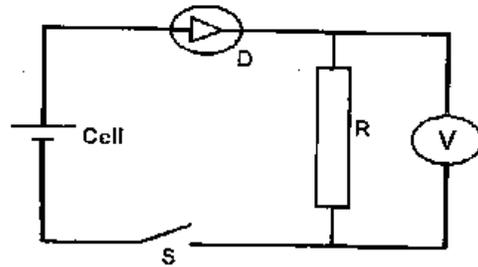
When the cell terminals are reversed and the switch is closed the voltmeter reading is zero. Explain these observations ( 3 marks)
