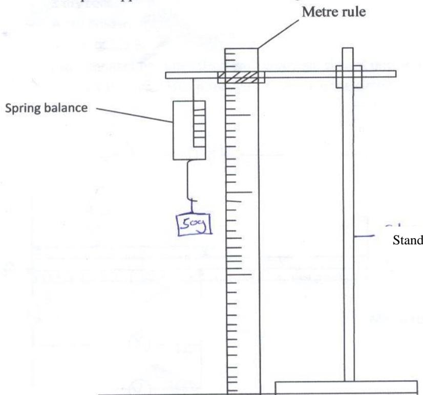
**b.** Hang 50g mass on the spring balance and note the extension and record your value in the table below. Increase the mass to 100grams and 150 grams noting the extension and recording it in the table.
