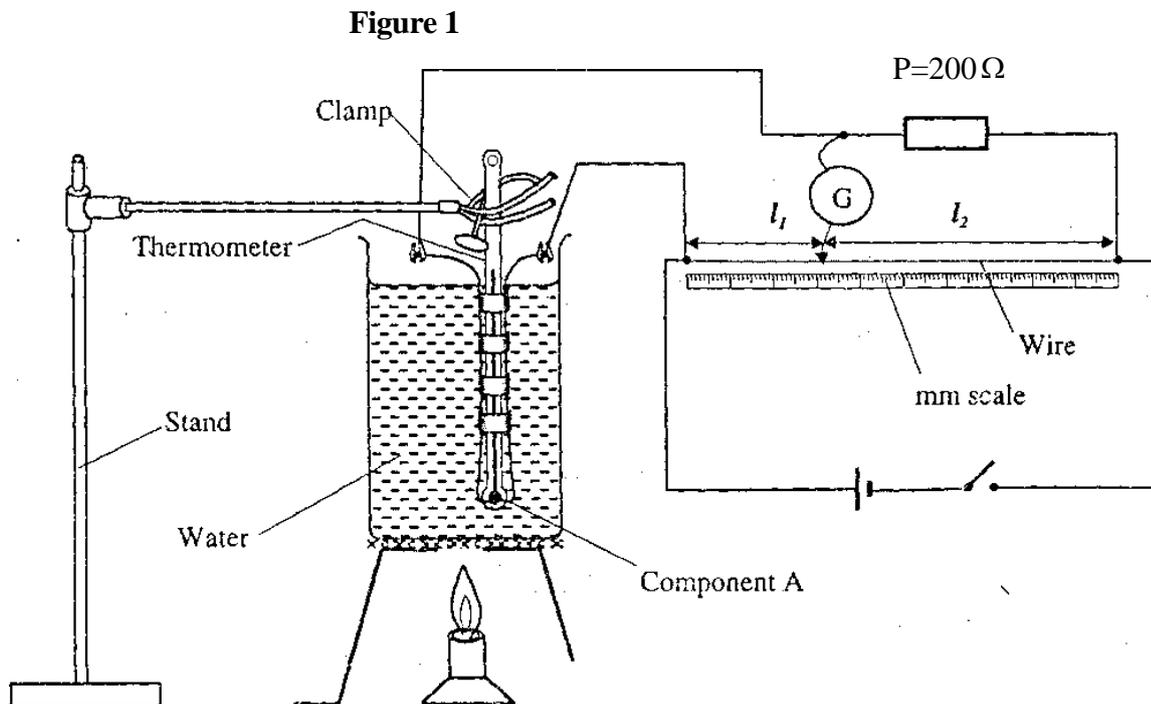
The thermometer and component A are mounted so that they do not touch the sides or the bottom of the beaker. The scale of the thermometer should face the candidate.
