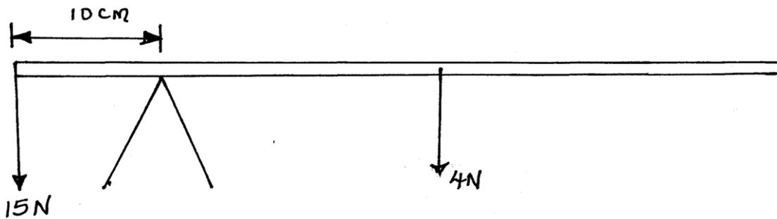
Given that the length of the bar is 0.5m, determine the weight of the bar. (2mks)
