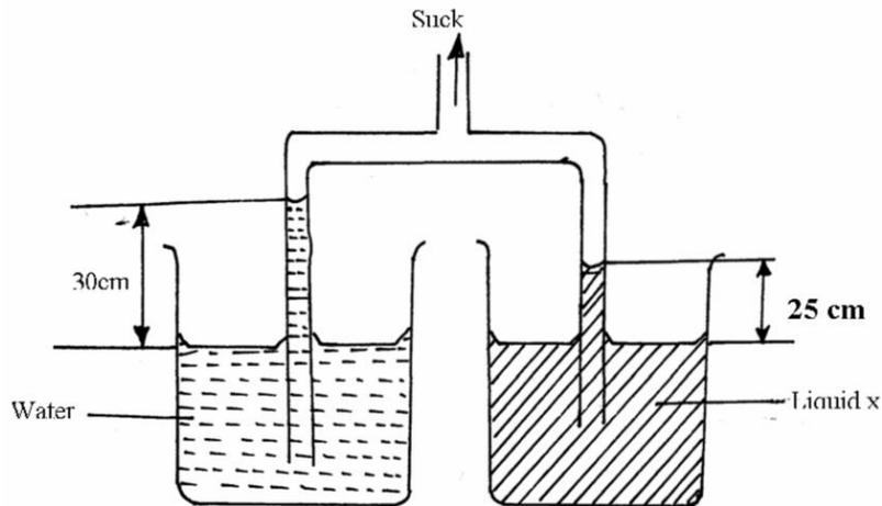
Use the information given in the above diagram to calculate the density of liquid x given that density of water is  $1000\text{kgm}^{-3}$ . (2mks)
