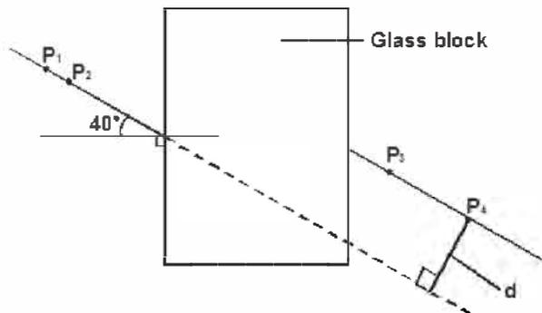
ii) Draw normal at point 2cm from the end of one of the longer side of the block outline. Draw a line at an angle of  $\theta = 40^\circ$  from the normal. Stick two pins  $p_1$  and  $p_2$  vertically on this line.
