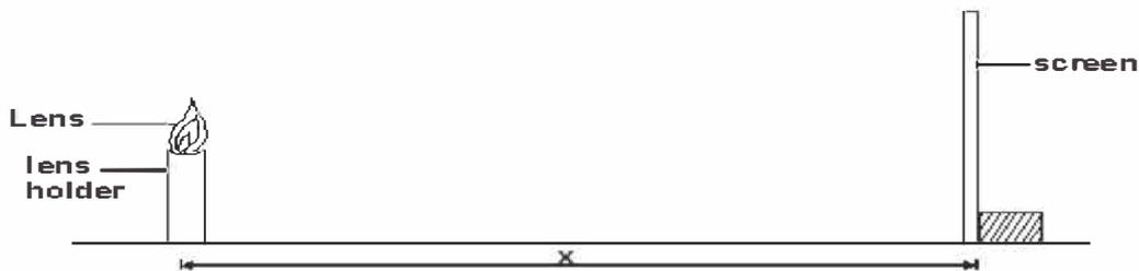
a) Measure the distance  $x$  in cm between the lens and the screen at which a sharp image is obtained repeat this two times, using different objects and record your readings in table 3 below.
